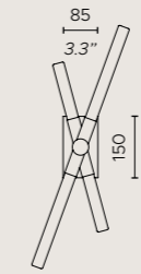
Con base - driver integrato With base - driver on board 110V version: supplied with plate to cover junction box
