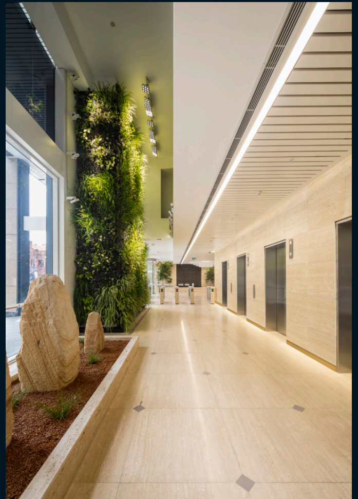
Bank of China, Sydney Stella wall-washers with an LED spectrum specifically tailored to the plants provide optimum light for the vibrant living wall in the foyer. Photography: Murray Harris Photography P/L, Artarmon.
