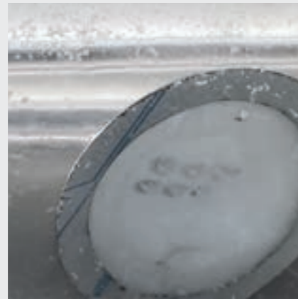
Low temperatures (-30°) resistance test
